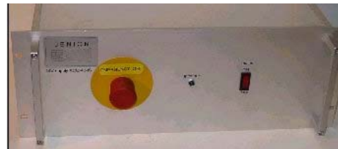
Fig.10: Optional Interlock- and main power interface
