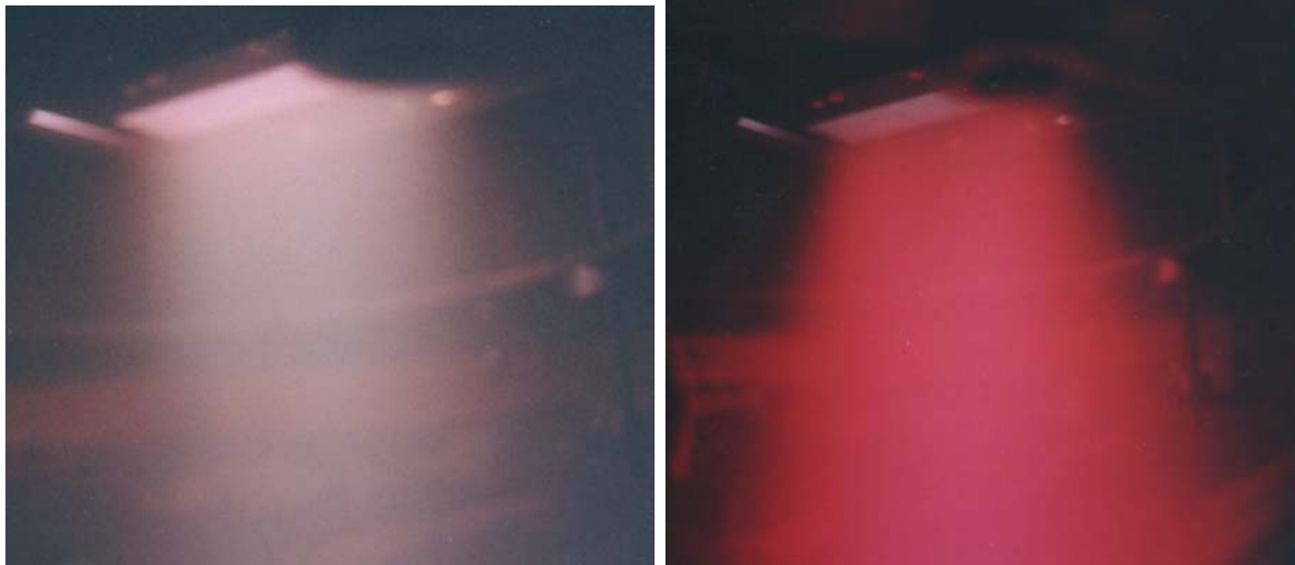
Fig.2: Ion source JENION ACC-30x125 IS in operation with oxygen (left) and hydrogen (right)
