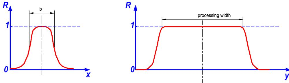
Fig.2: Typical plasma or beam profiles of linear plasma or ion beam sources (normalized deposition or etch rate R)
