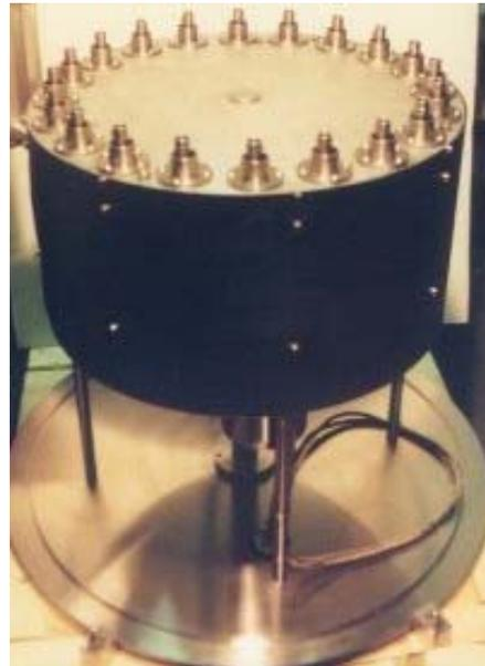
**Fig.5:** Customer specified high voltage substrate holder for max. 20 kV Substrate bias with two integrated stepper motors for independent substrate rotation
