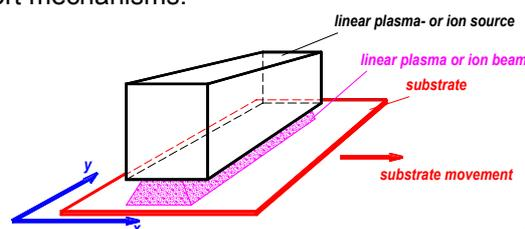
**Fig.1:** Principle of processing with linear plasma- or ion beam sources
