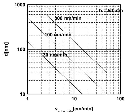
Fig.3: Processed thin film thickness in dependence from the substrate velocity and the thin film deposition rate of the plasma- or ion beam source with the process width of b= 50 mm (calculated after (1)).
