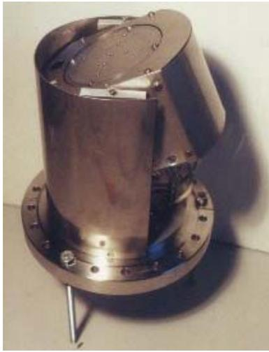
**Fig.4:** Customer specified flange mounted inside heated substrate holder for max. 100 mm diameter with substrate rotation and angle movement by two integrated stepper motors
