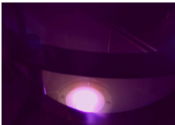
Fig. 2: Plasma source ACC-80 PS in operation with nitrogen
