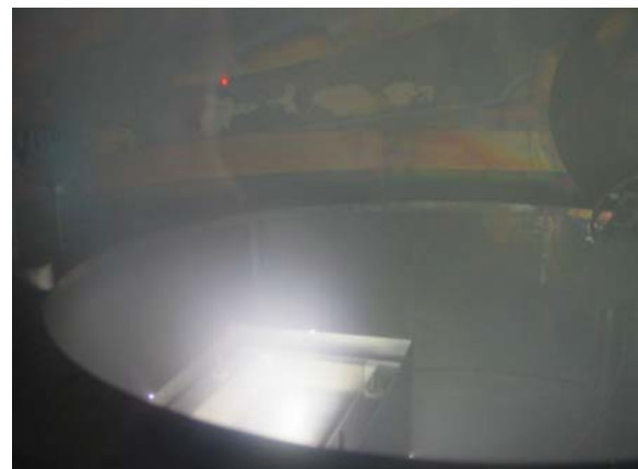
Fig. 3: Linear plasma source ACC-40x150 PS in operation with oxygen ( 4 \times 10^{-4} mbar, I_{\text{plasma}} = 0.25 A),
