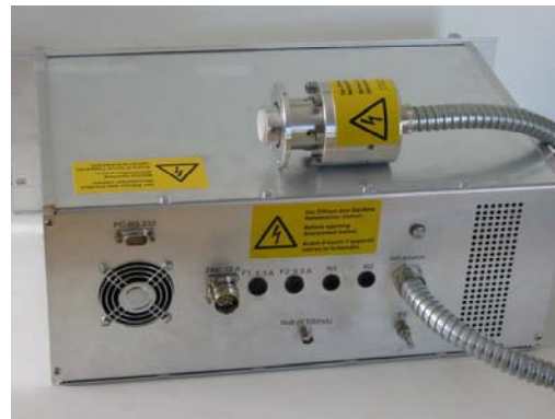
Fig.10: Electronic Control unit (back side with ion source connector cable)
