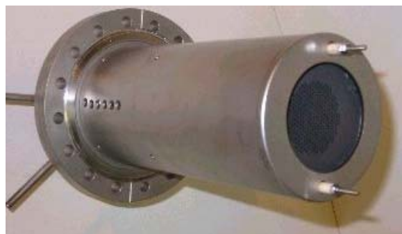
Fig.1: Ion source JENION ACC-40 IS (left), and in operation
